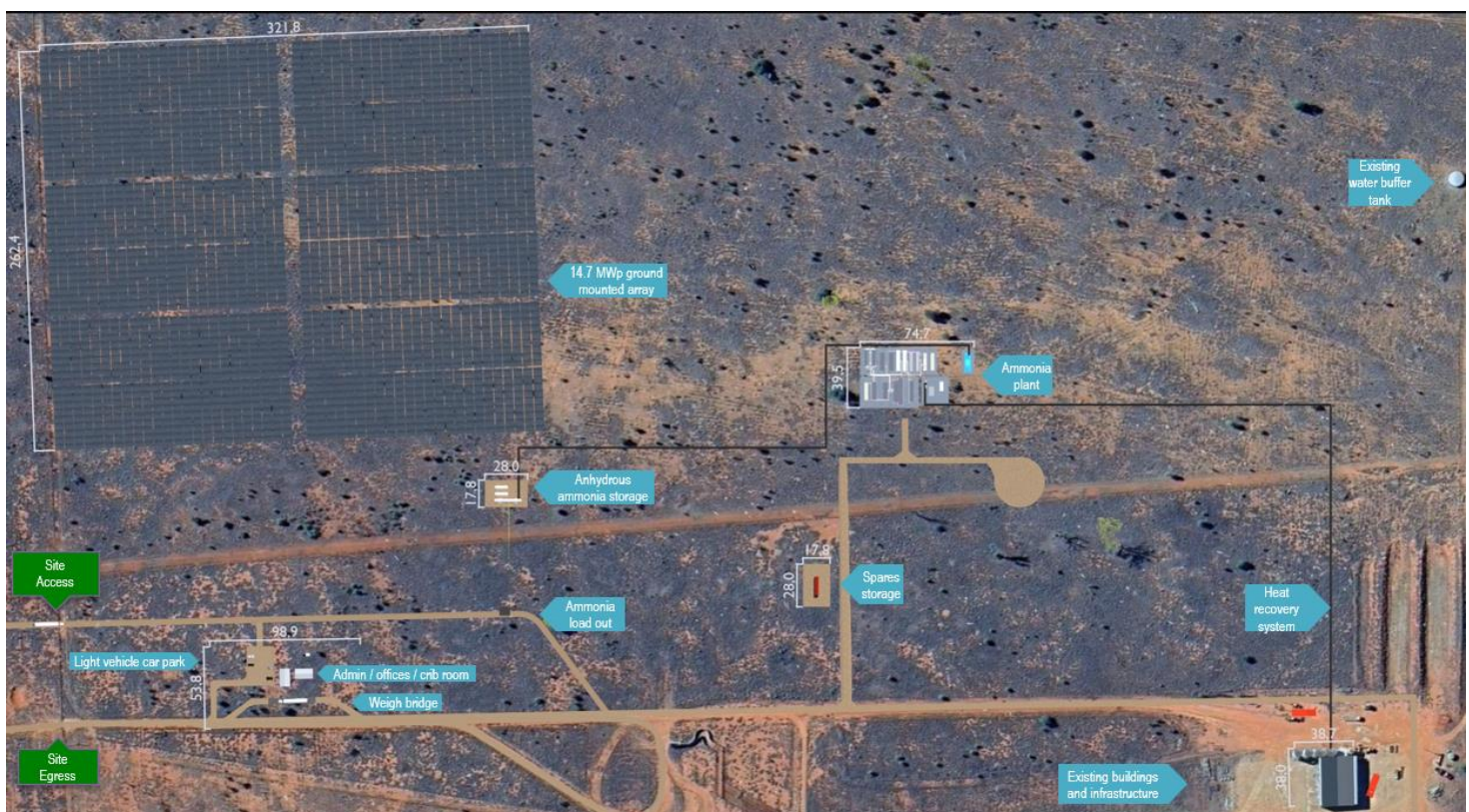
Figure 11: Site plan view. The footprint of the facility is 447m x 625m (28 Ha), with most of this surface area being the solar array or buffer space between the elements of the facility. A higher resolution site plan view is provided as a separate document.
